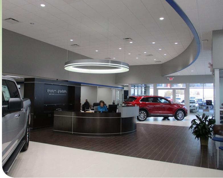
*Vive controls ensure the proper lighting on the cars at all times — 150-200 fc during the day, and 75 fc at night when many customers like to window shop.*
